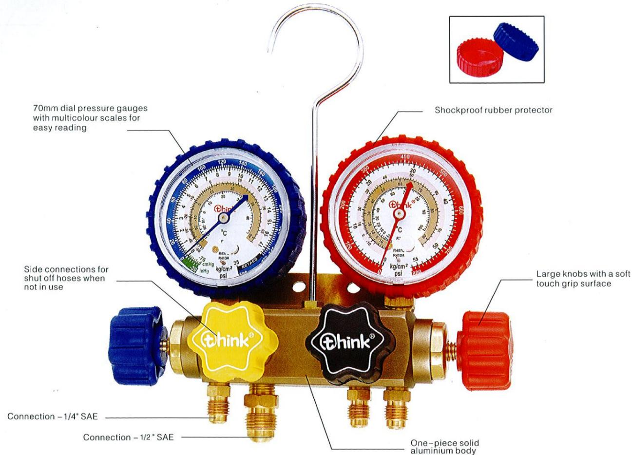
4-WAY ALUMINIUM TESTING MANIFOLD WITH PISTON VALVE FOR R410A
