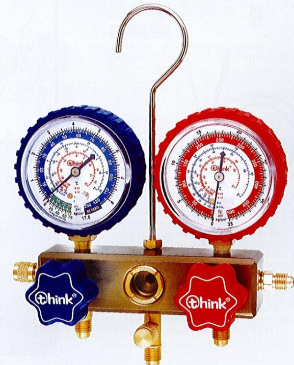
FOR R134A BRASS TESTING MANIFOLD
