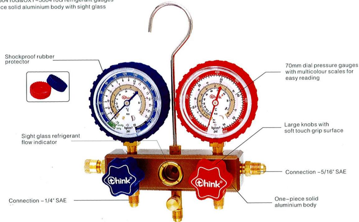
2-WAY ALUMINIUM TESTING MANIFOLD WITH SIGHT GLASS FOR R134A
